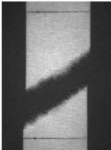
Fig. 4. Example of a localized failure zone in a sample with a_1 = 0.0 . The high level of fiber pull-out is apparent.
